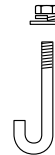
Detail of the "J" Bolt and Hardware shipped with the RAIL RIDER ™ Adapted Slider Base
