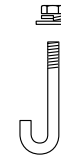
Detail of the "J" Bolt and Hardware shipped with the RAIL RIDER™ Adapted Slider Base
